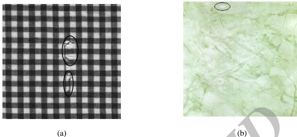
Figure 1. An example of a defective regular texture (a) and a defective random texture (b). The defects of each image have been marked by elliptical lines.
