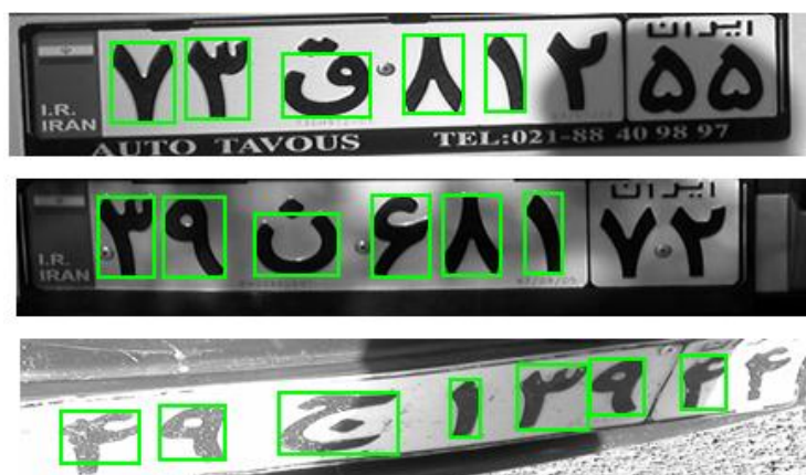
Figure 8. Unsuccessful character segmentation using the proposed segmentation method
