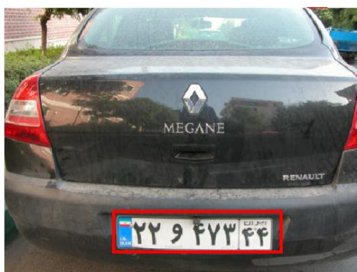
Figure 4. Recognition of the entire license plate using the blue margin
