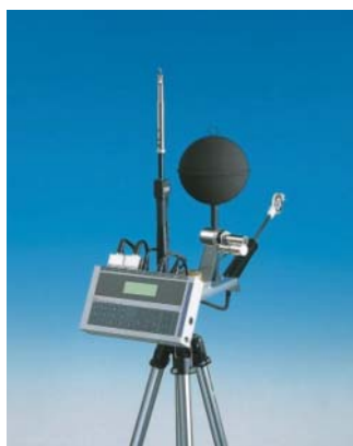
Fig. 1: The data acquisition System BABUC and two examples of microclimatic measurement (winter and summer – Indépendance square)
