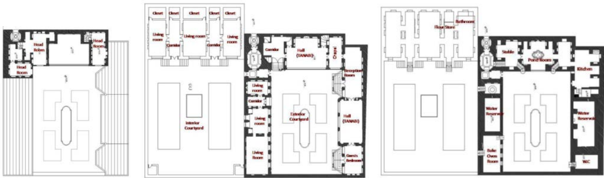
Fig.6: Plans of the Salmasi House complex, from right: basement, ground floor, first floor
