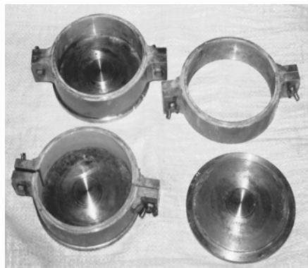
Figure 3 Mould with specimen and demoulded mould (steel ring)
