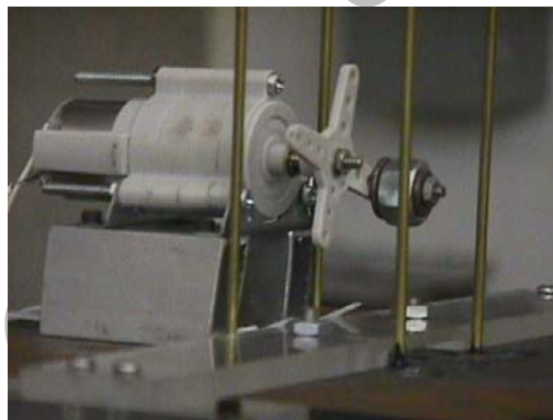
Figure 2 Excitation motor with eccentric mass
