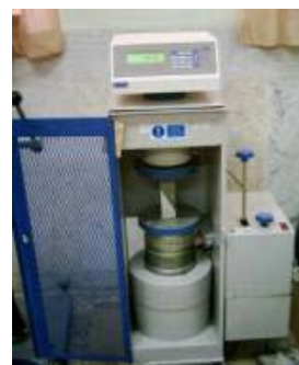
Figure 2. Slant shear test
