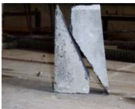
Figure 1. Concrete samples prepared based on BS 6319: Part 4
