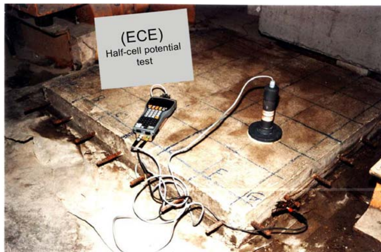
Figure 7. Half-cell potential instrument
