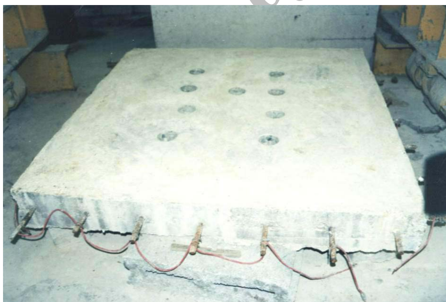
Figure 3. Pattern of core drilling in slab
