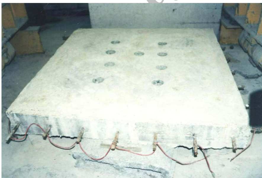
Figure 3. Pattern of core drilling in slab
