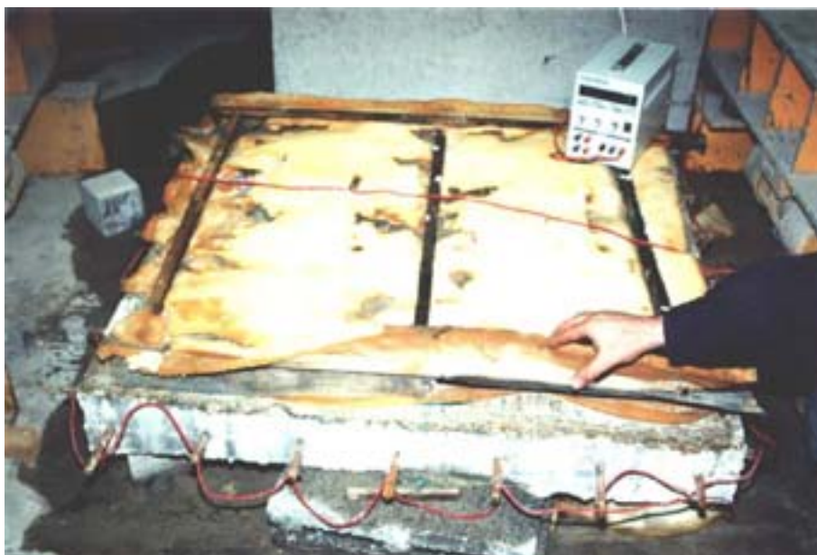
Figure 2. Equipment and application of electric field
