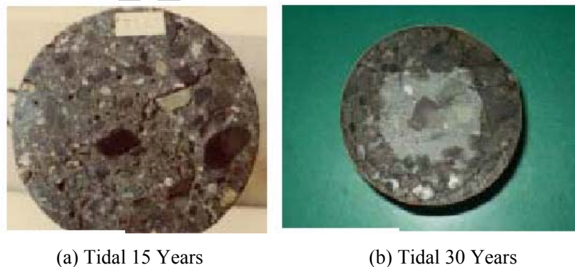
Figure 3. Transverse section of the tidal specimens
