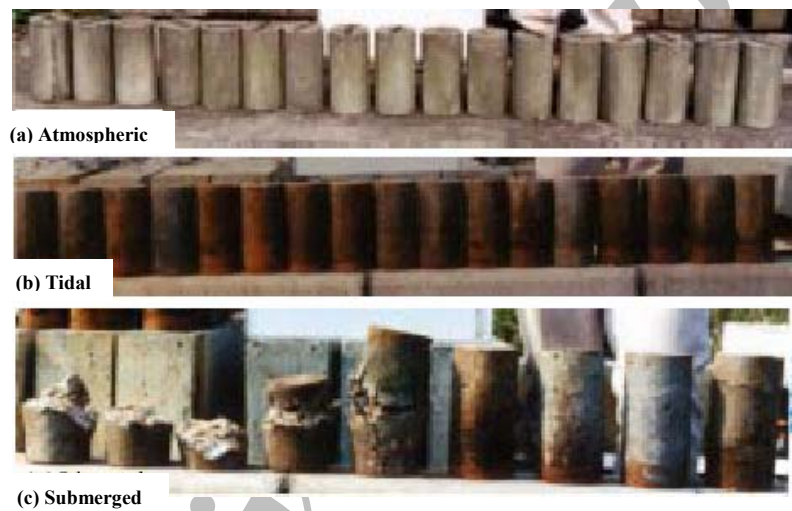
Figure 2. Appearance of some specimens (at 15 years of exposure)
