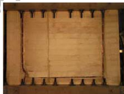
(b) SRF-A: Strengthened with conventional detail
