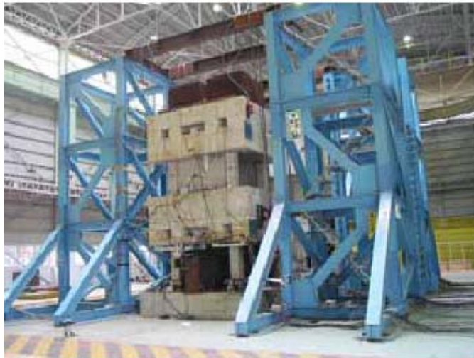
Photo 2. Eccentric pilotis frames on the shaking table at NIED
