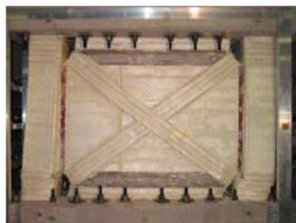
(c) SRF-X: Strengthened in the new detail
