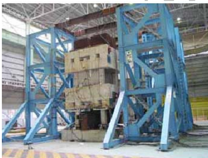
Photo 2. Eccentric pilotis frames on the shaking table at NIED
