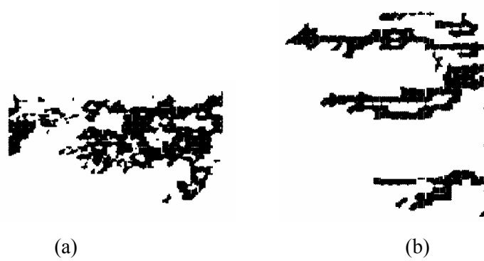
Figure 4. Flow patterns obtained from volume of Fluid model with different injection flow rates
