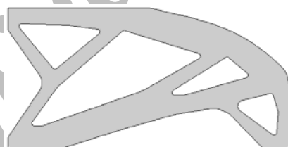
Figure 9. CAD model of the obtained optimum layout by using cellular automata technique
