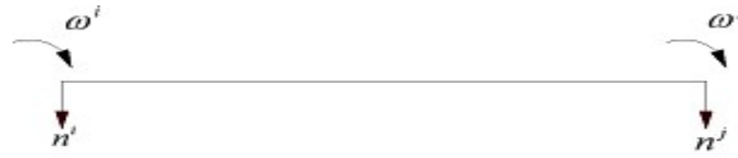
(a) Sign convention for member displacements. Directions as shown are considered positive
