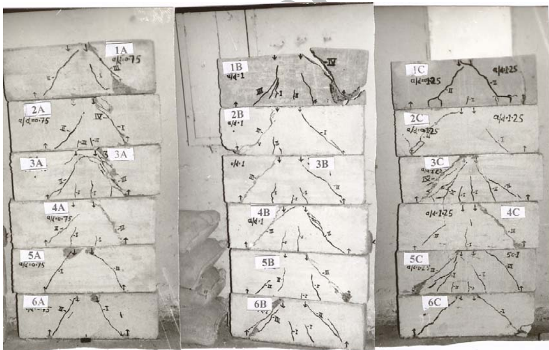
Figure 4. Cracking pattern and mode of failure for tested beams
