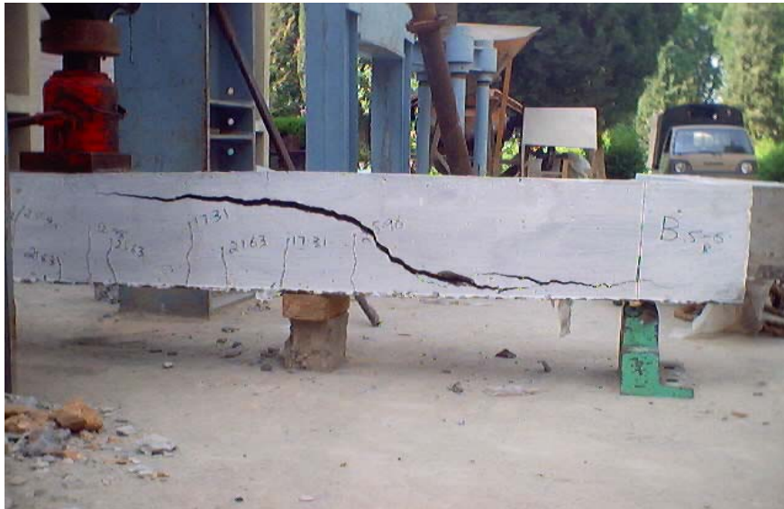
Figure 6. Typical shear failure of slender beam without web reinforcement at \rho > 1\% ( \rho = 1.5\% a/d = 5.5 , Span = 203cm)
