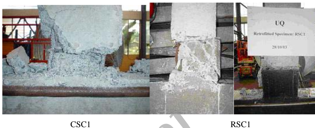
Figure 11. Failure pattern of specimens CSC1 and RSC1.
