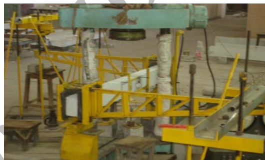
Figure 5. Torsion test rig along with twist meter
