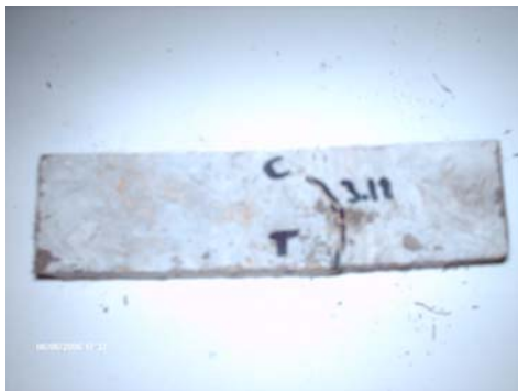
Figure 12. Prewetted diss fibres composite, W/C=0.7 ratio, after flexural test
