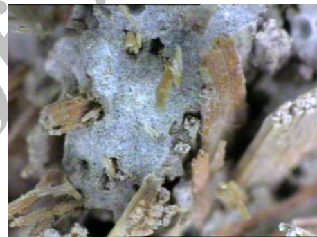
Figure 13. Video microscope image on the crack, magnification×50
