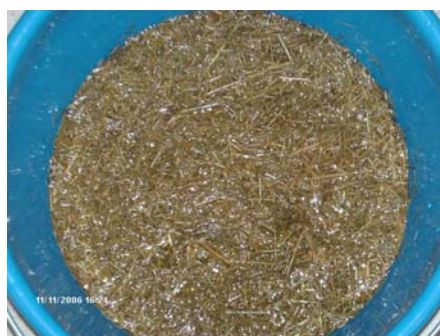
Figure 11. Saturation of Diss fibres during 1 hour
