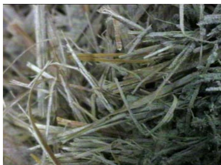
Figure 6. Video microscope image on the crack of unboiled diss composites, magnification x 25
