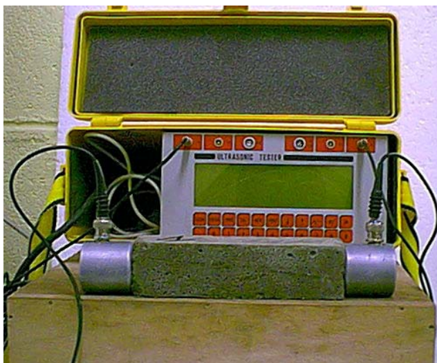
Figure 1. Standard E0641 Ultrasonic test setup
