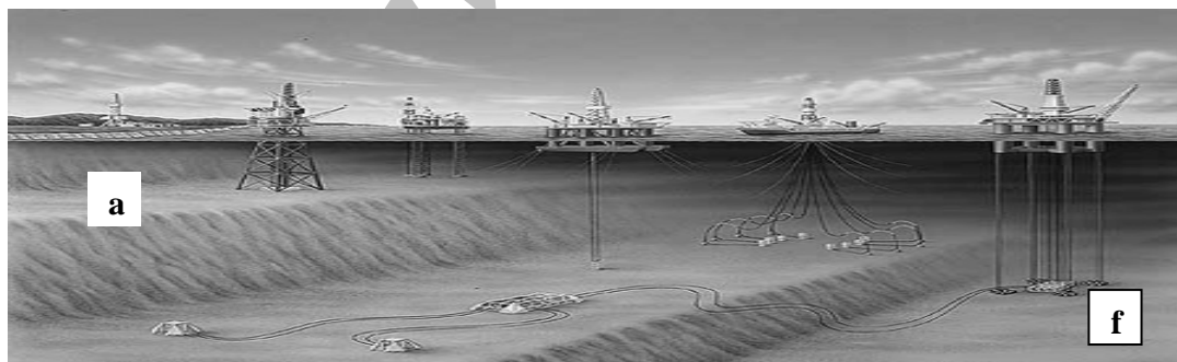
Figure 1. (a) Onshore platform (b) Fixed platform (c) Jackup rig (d) Semi-submersible (e) Drill ship (f) Tension leg platform
