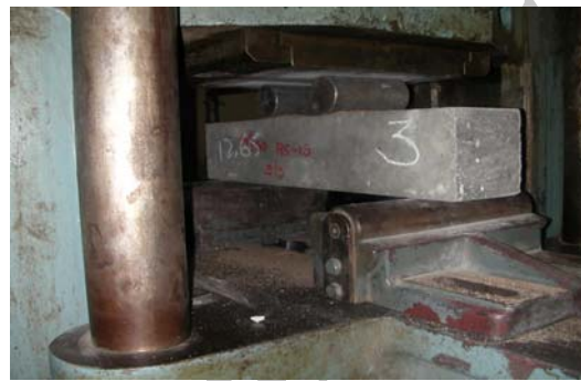
Plate 4. Test for flexural strength of Concrete
