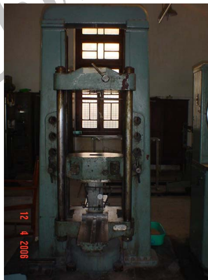
Plate 5. Test setup for Stress –Strain Curve of C
