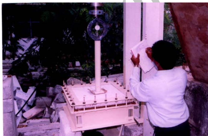
Figure 3. Testing of slabs for punching shear
