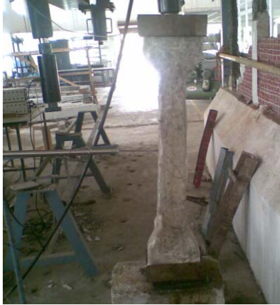
Figure 7. Experimental set up for wrapped short column
