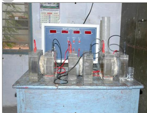
Figure 2. Chloride ion permeability test setup
