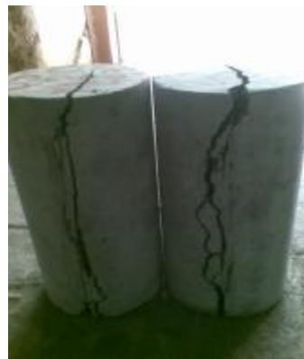
Plate 4. Cracking pattern of cylinders
