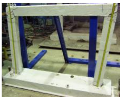
Figure 3. The BF model after pushover testing and its pushover curves
