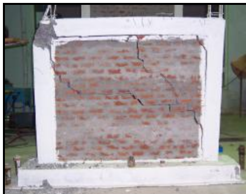
Figure 4. The IBF model after pushover testing and its pushover curves
