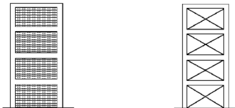
Figure 10. Re-evaluation of seismic capacity of 4-storey RC frame with infill wall and steel bracing
