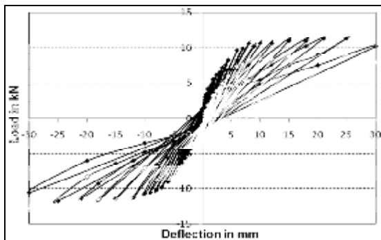
Figure 12. Hysteresis curve for monolithic specimen ML
