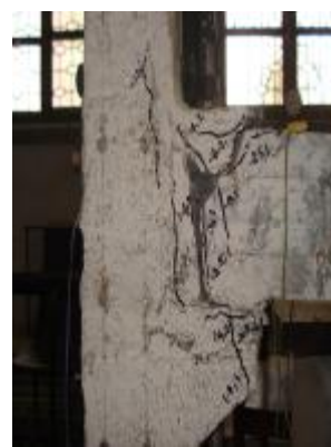
Figure 11. Failed cleat Angle connection
