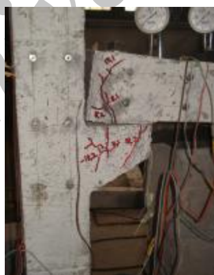
Figure 10. Failed J-bolt connection
