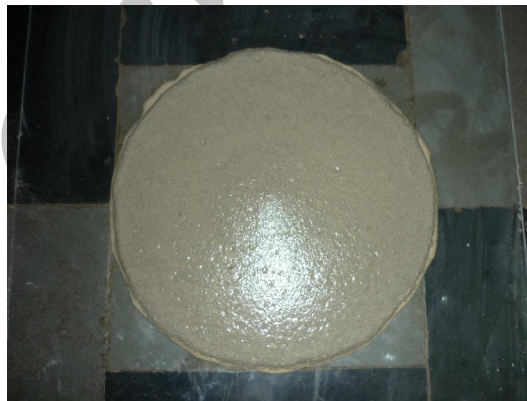
Figure 6. Spread with halo of the Mix 2 at 0.7% SP
