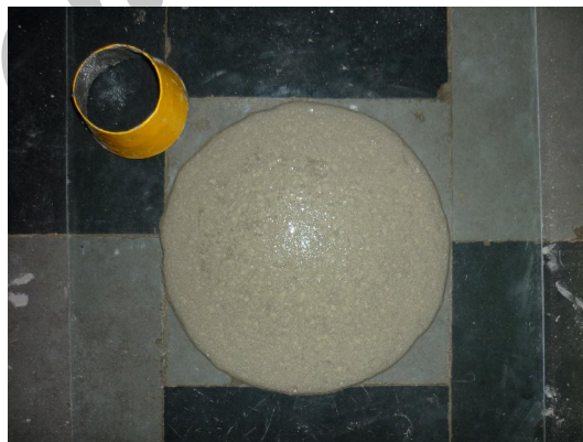
Figure 8. Maximum spread of the Mix 2 at 0.9% SP and 0.2% VMA
