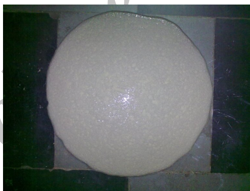
Figure 5. Maximum spread of the Mix 1 at 0.9% SP
