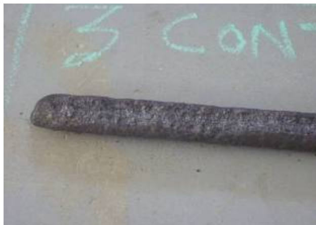
Figure 11. Typical view of cleaned rebar and view of reduced cross section
