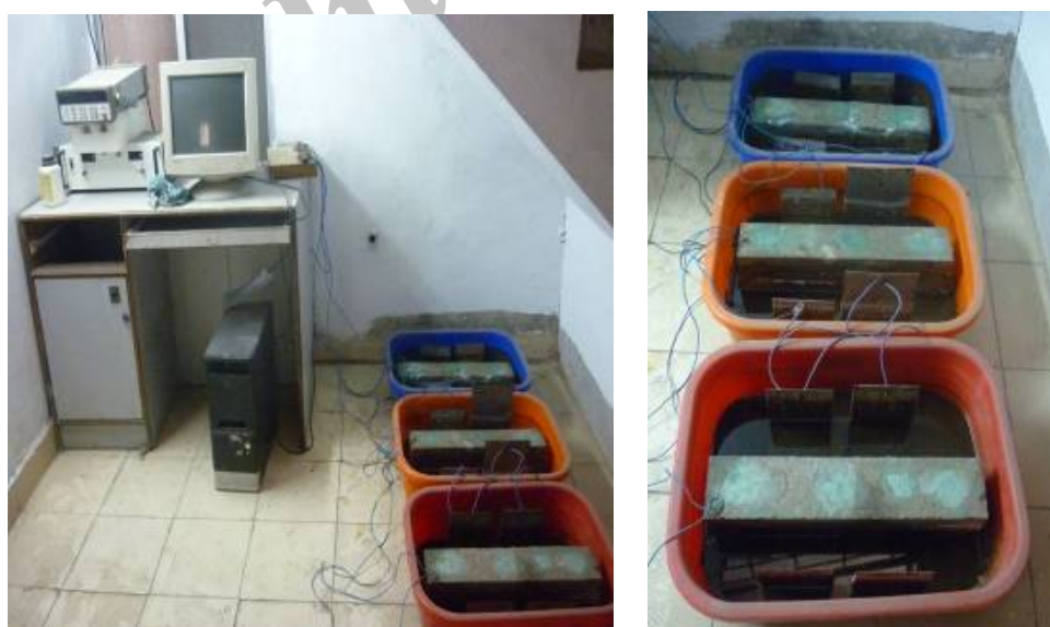
Figure 7. Typical view of accelerated corrosion setup
