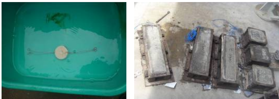
Figure 6. Specimen preconditioning & concreted with required wires
