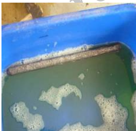
Figure 11. Typical view of cleaned rebar and view of reduced cross section
