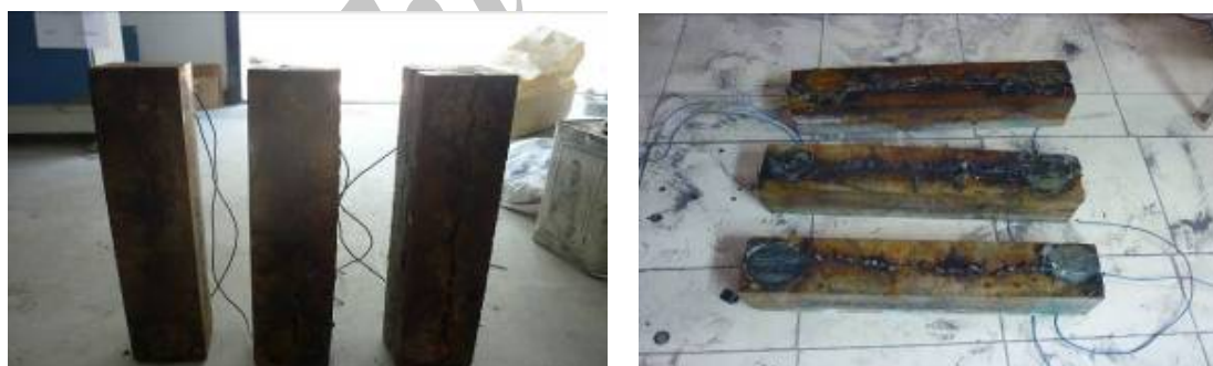
Figure 8. Typical view of corroded specimen
