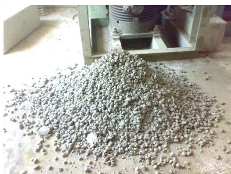
Figure 2. Fresh geopolymer concrete ready to use
