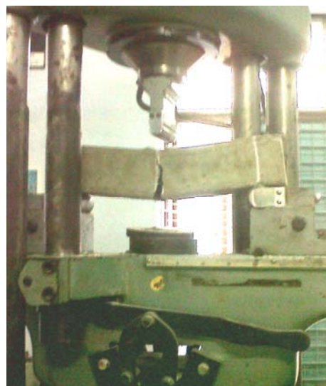
Figure 6. Typical flexural strength test set up after test
