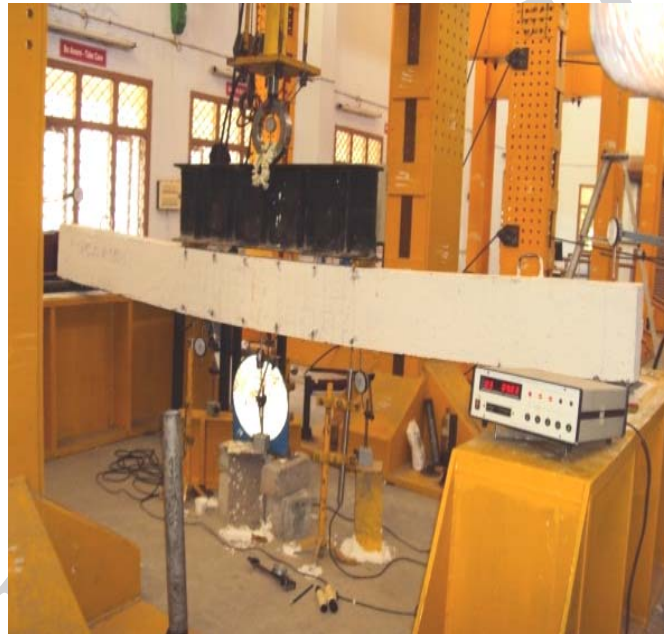
Figure 4. Loading set up
