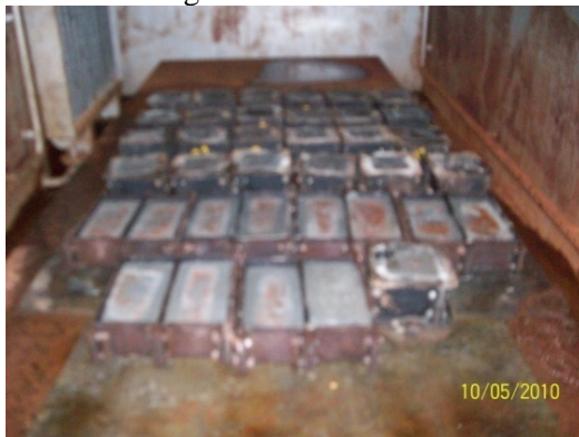
Figure 4. Steam curing of geopolymer bricks
