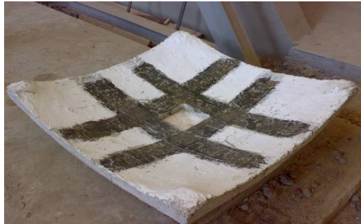
Figure 4. Shell "SOG1" strengthened using 2-layers of GFRP wrap (Type 1).
