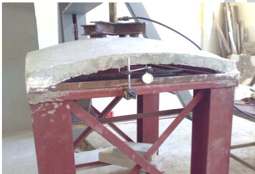
Figure 7. Shell strengthened by using external tie "SOT".
