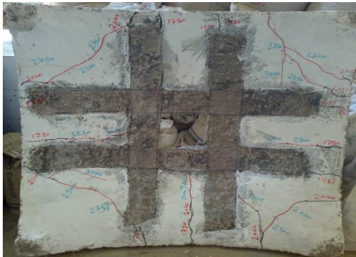
Figure 26. Crack pattern of shell "ROG1" repaired by using 2 layers of GFRP (Type 1). [Failure load = 3000 kg]
