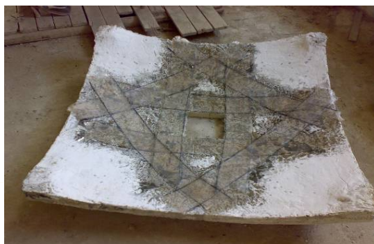
Figure 6. Shell "SOG3" strengthened using 2-layers of GFRP wrap (Type 3).
