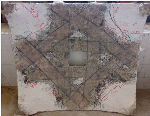
Figure 24. Crack pattern of shell "SOG3" strengthened by using 2 layers of GFRP (Type 3). [Failure load = 3500 kg]
