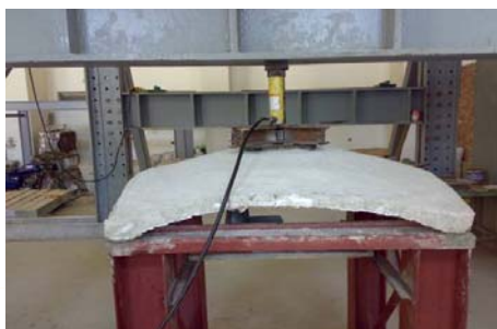
Figure 3. The arrangement of the hydraulic jack which applying the load.
