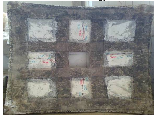
Figure 23. Crack pattern of shell "SOG2" Strengthened by using 2 layers GFRP (Type2). [Failure load = 3500 kg]
