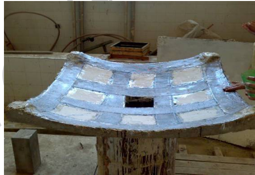
Figure 5. Shell "SOG2" strengthened using 2-layers of GFRP wrap (Type 2).
