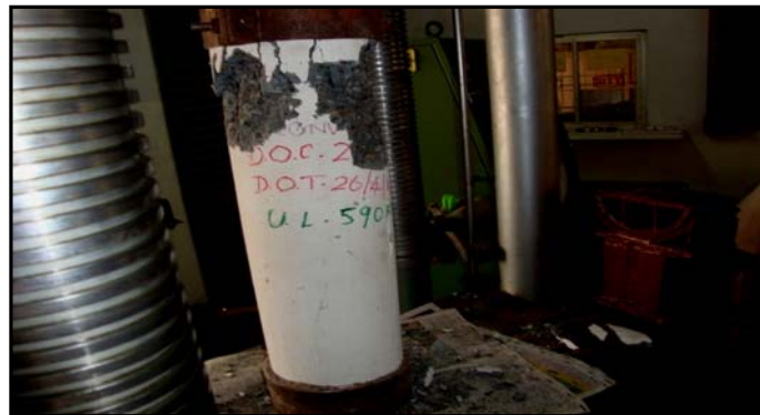
Figure 4. Failure pattern of plain RC column
