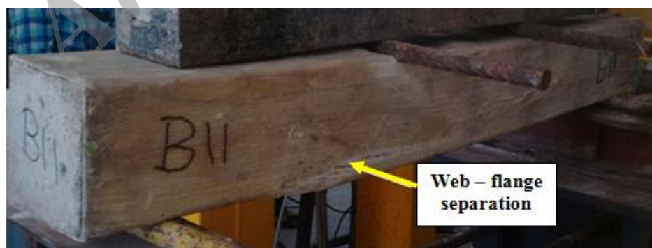
Figure 10. NSC infilled UDC GFRP tubular beams (R2U)
