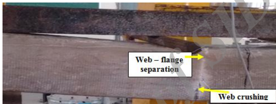
Figure 12. Hollow WR GFRP tubular beams (RW)
