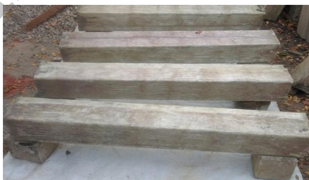
Figure 5. Concrete filled GFRP thin walled tubular beams
