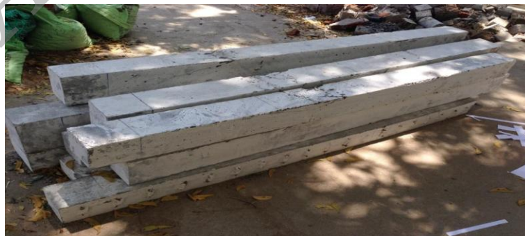
Figure 9. Picture showing 9 nos. of specimens after Ultimate Loading
