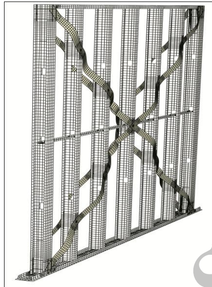
Figure 4. Deformed shape of the FE model after 110 s
