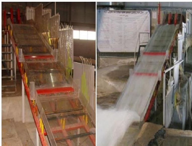
Figure 1- The Physical Model of Free dam spillway
