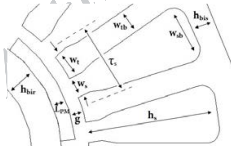
Fig.1 Motor topology showing geometrical definitions
