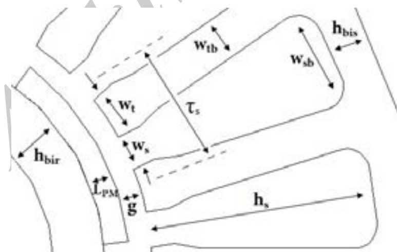
Fig.1 Motor topology showing geometrical definitions
