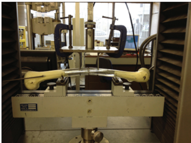
Figure 1: Loaded femur stabilized with titanium nails
