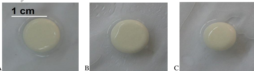
Fig. 4: Photographs of a tablet made of HPMC 100K:HPMC 4000 (1:1) during dissolution in simulated gastric fluid (SGF) after; A) 30 min, B) 60 min, and C) 180 min.
