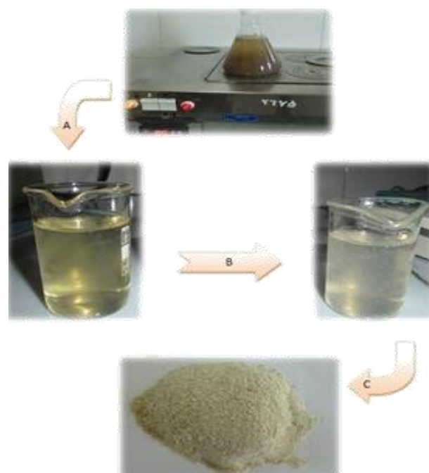
Figure 2. Procedure of psyllium gel extraction. A) psyllium gel and seed were separated from supernatant. NaOH was added to dissolve psyllium gel; alkaline solution was separated from the residue by centrifugation. B) Alkaline solution was neutralized by HCl 2M. C) White gel was harvested by centrifugation from supernatant; dried and grinded.
