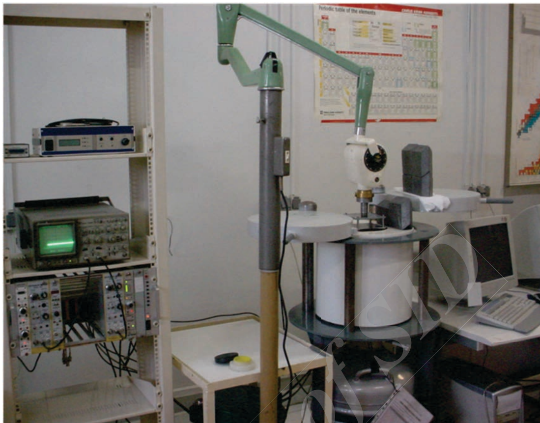
Figure 3. The picture of measurement setup including X-ray tube, collimators and a semiconductor detector (HPGe).
