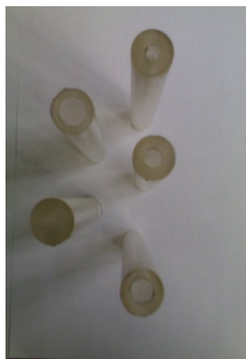
Figure 4. PMMA cylinders with 20 mm diameter
