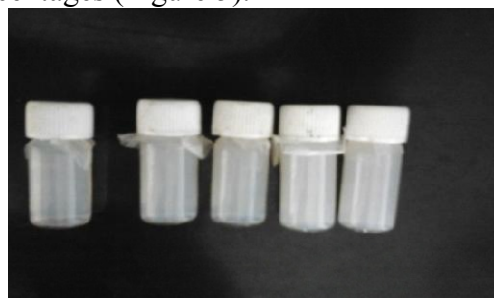
Figure 5. Gels made with different percentages of hydroquinone, from left: 3%, 2%, 4%, 5% and 6%.
