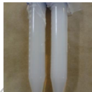
Figure 4. Irradiated tubes (left: 0 Gy, right: 15 Gy)
