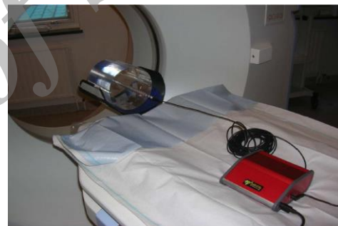
Figure 2. CTDI phantom and pencil dosimeter chamber [8]
