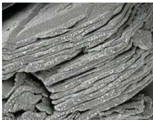
Figure 3: Nanoparticles of three calcium aluminate ( 3\text{CaO}, \text{Al}_2\text{O}_3 )
