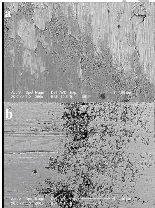
Fig. 9. SEM micrographs of surface of coated sample following abrasive wear with 355-425 \mu\text{m} silica-rubber wheel as a function of environment: (a) dry-plan view (b) wet-plan view.
