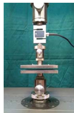
Figure 2: Universal testing machine for testing the compressive strength of the samples
