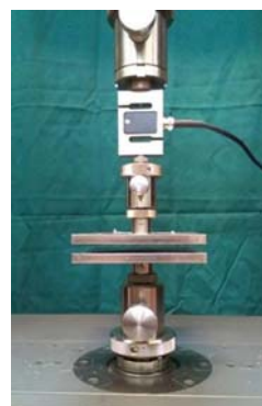
Figure 2: Universal testing machine for testing the compressive strength of the samples
