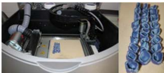
Figure 4: Wax-patterns fabricated by RP technology
