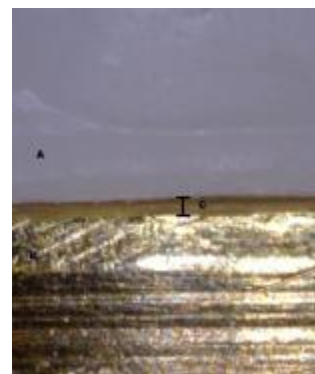
Figure 3: Captured image of coping-die interface (Zirconia coping (A), Brass master die (B), marginal gap (C))
