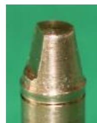
Figure 1: Brass master die
