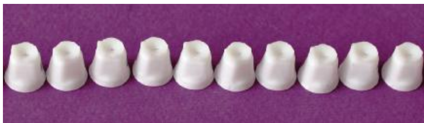
Figure 2: Fabricated zirconia CAD/CAM copings
